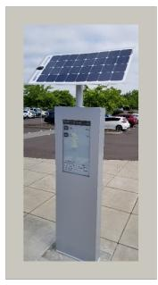
SMART's new eReader Console, installed at the end of May at the Transit Center, is solar operated and provides riders with real-time information on bus arrivals and departures. The 32" screen allows for customization such as rider alerts and event details. The system can be expanded to other, smaller, eReaders at SMART's busiest bus stops as funds become available. The new Console was purchased utilizing FTA Section 5307 formula funds.
